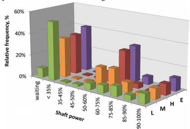
Fig. 5. Power level pattern of leader-type icebreaker over typical year of operation in light (L), medium (M), heavy (H) and extreme (E) ice conditions.
