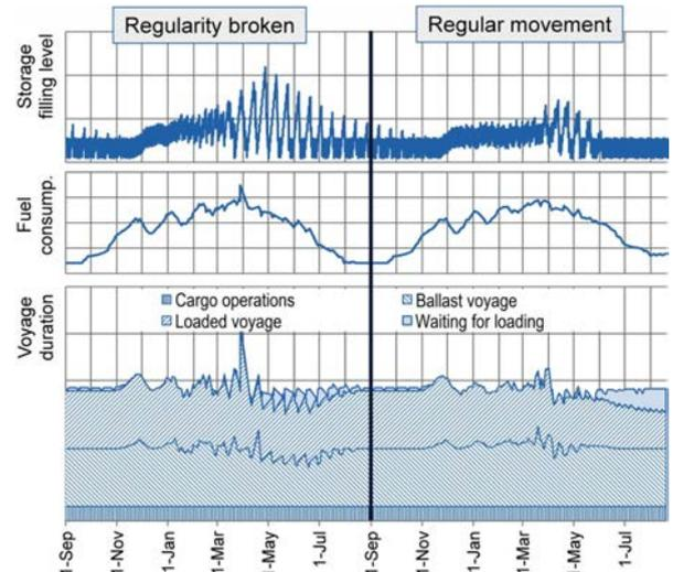
Fig.11. Influence of regularity of tanker movement on operational parameters of the system
