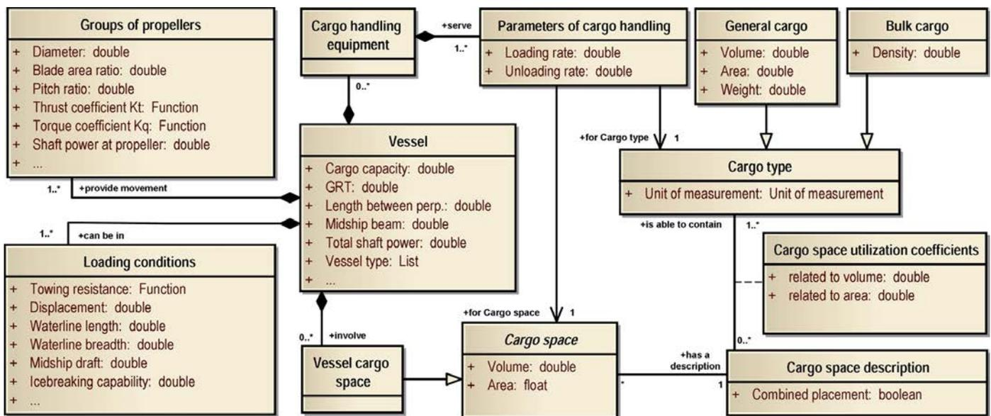
Fig. 1. Class diagram of ship & cargo object model in UML notation (part of general model)
