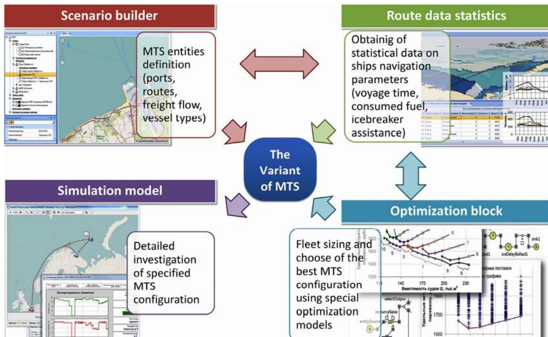
Fig.4. Layout of the software blocks for MTS investigation
