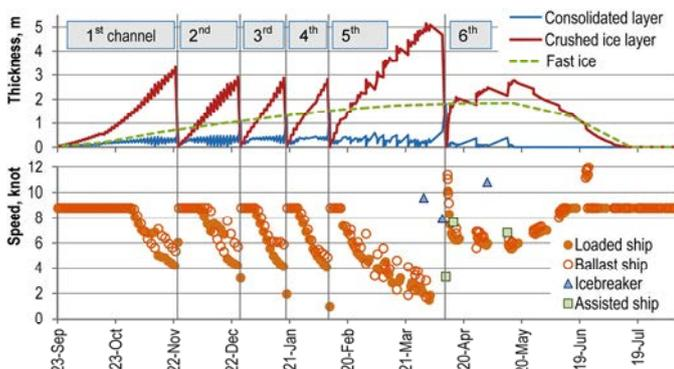
Fig.10. Parameters of ice channel segment near Novy Port in heavy ice conditions.
