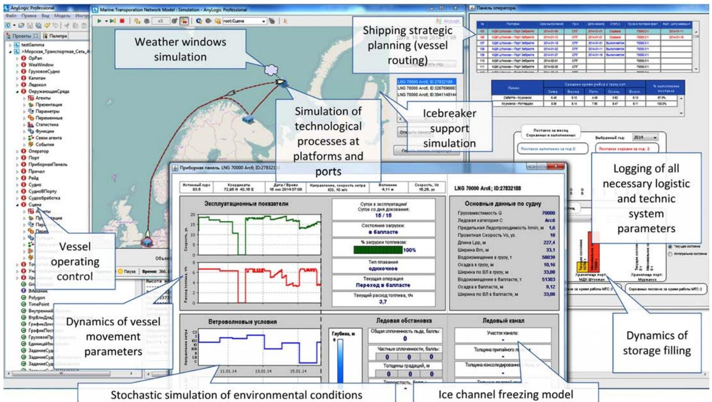
Fig.3. Agent-based simulation model of marine transport system and main simulated processes.
